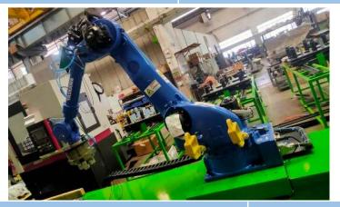
Lokesh VTL with Yaskawa Robot with Auto Gauging 3Machines Cell
